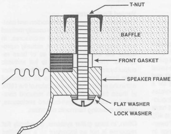
**FIGURE 5 — Button-Head Machine Screw for Front Mounting (not to scale)**
