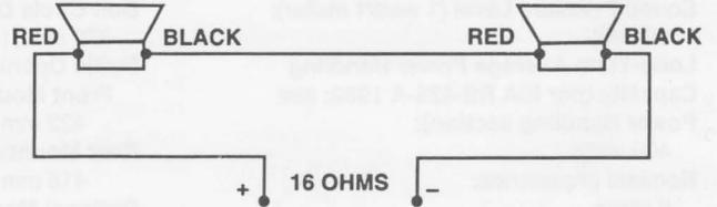
**FIGURE 8 — Connection of Four 18BX Speakers in Series/Parallel (net impedance is 8 ohms)**
