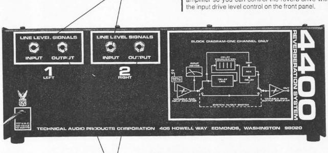
**OUTPUT CONNECTORS:** ¼" phone plugs are also used for the output connectors to facilitate hook-up ease. These are line level outputs, capable of 10 volts RMS into a 5000 ohms or greater load. Signal strength is controlled by the output level controls on the front panel.
