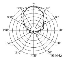
Figure 6—Beamwidth vs. Frequency (anechoic environment)
