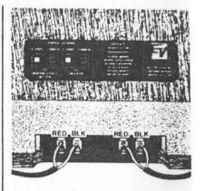
crossover) by 3 dB and leaving the Environment control in the 1/4 Space position. The 3 dB attenuation may be evaluated by ear, although the most accurate setting will be obtained if the system is driven with a sine wave whose frequency is above the 350 Hz crossover (say, 1000 Hz) and the galn reduction is measured with an appropriate AC voltmeter placed on the output of the high-frequency power amplifier.
