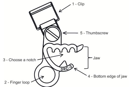
2. Choose a notch (3) at the top of the DRC-2 jaw and place it to the drum rim so the top edge of the rim fits inside the desired notch.
