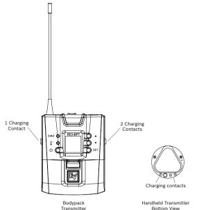
Transmitter charging contact locations are as shown. A bodypack transmitter contains three contacts; one on the left side, and two on the right side. These must align with the single and dual contacts of the charger slot. The handheld transmitter contains three charging contacts located toward the tail end of the transmitter; one on the left side, and two on the right as shown. These must align with the single and dual contacts of the charger slot.
