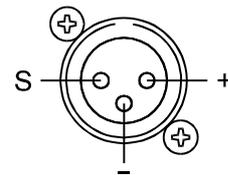
Pin-assignment of the “PHOENIX”-type connectors:
