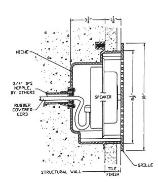
Figure 1 Typical Installation of a KDI Paragon Wet-Niche #68102
