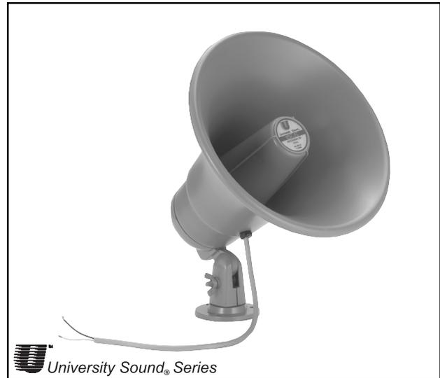
The mounting base shall provide orientation adjustment in all three planes. Vertical adjustments are made by loosening a single wingnut on the mounting base.
