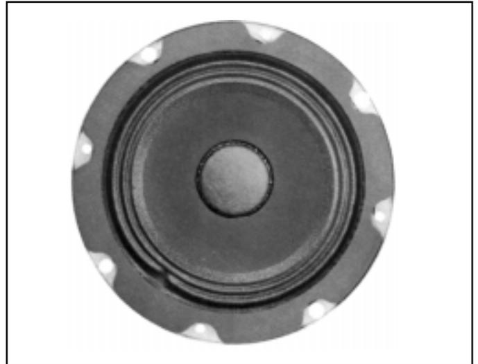
reference efficiency shall be 0.8%. The nominal impedance shall be 8 ohms and the dc resistance shall be 6.5 ohms. The loudspeaker shall be capable of handling a continuous 10-watt (8.6 volts true RMS) shaped white-noise signal (as per EIA Standard RS-426A 1980) with a 6-dB crest factor for eight hours.
