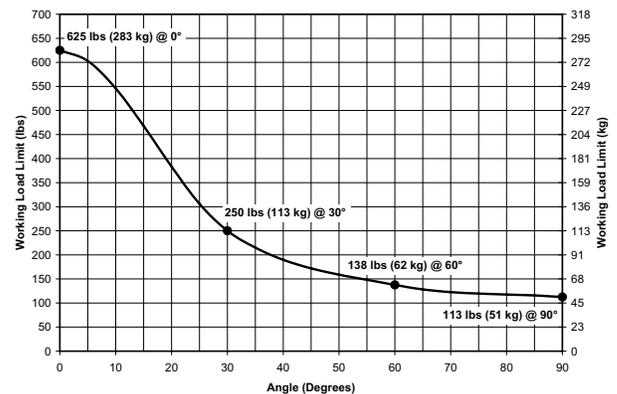
Table 2: Working-Load vs. Angle (8:1 Safety Factor)
