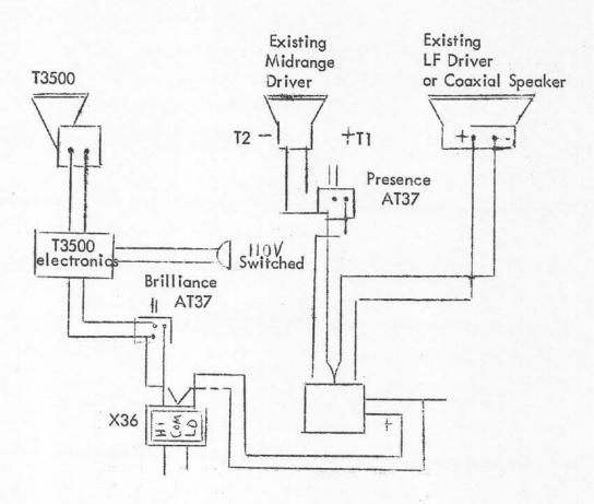
Figure 2 - Addition of Ionovac Driver (BB6)
