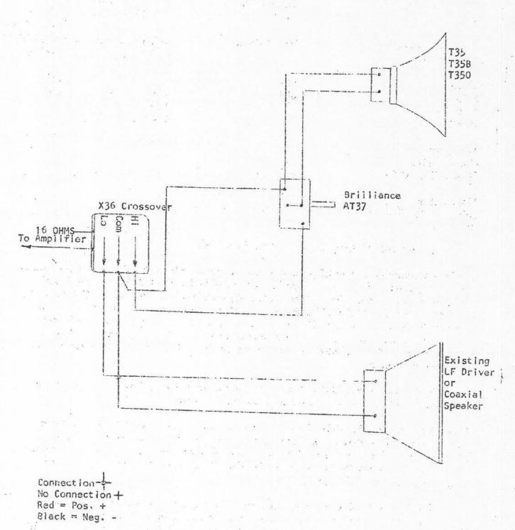
FIGURE 1 - Addition of VHF Driver (BB-5)
