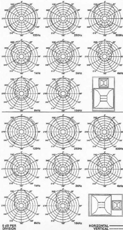
FIGURE 4 — MTH-2.5/64BT Beamwidth vs. Frequency
