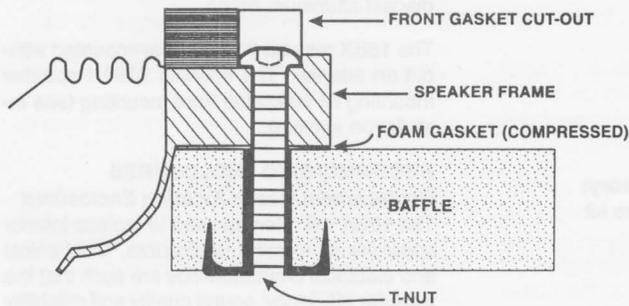
**FIGURE 4 — Rear-Mounting Detail (not to scale)**
