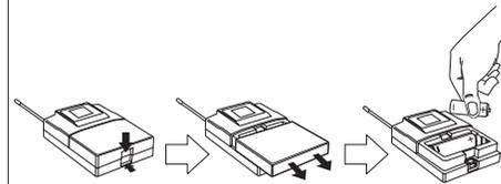
7. Install Batteries in Transmitter
