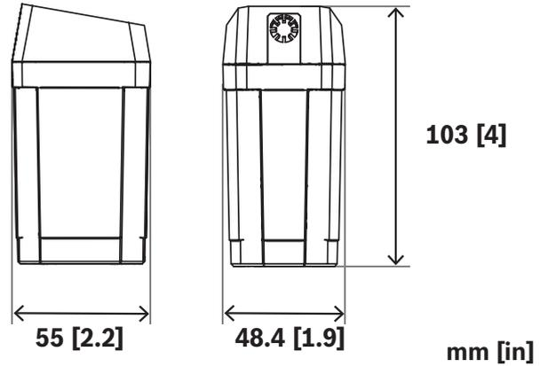
Fig. 3: Subwoofer adapter for EVOLVE-WMK with Phoenix-style connector
