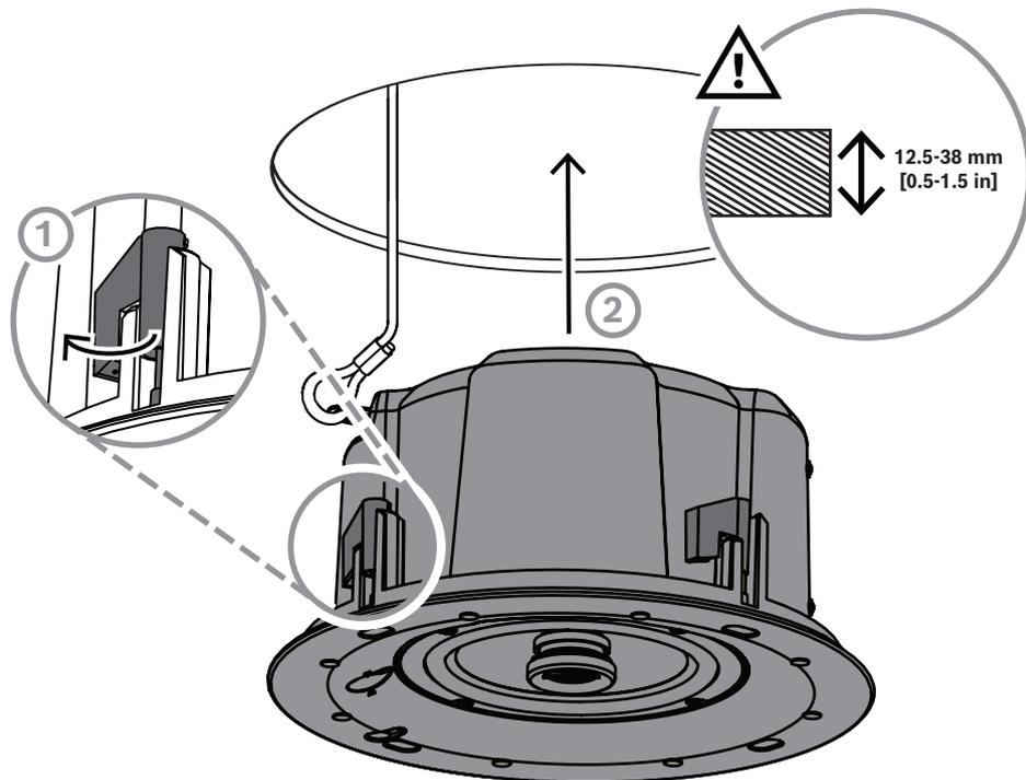
**Figure 4.6:** Mounting the speaker into the ceiling
