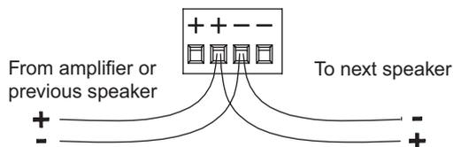
**Figure 4.3:** Parallel wiring
