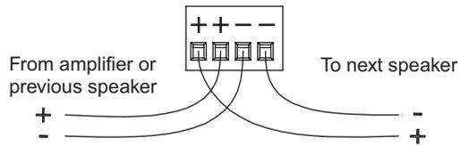
**Figure 4.4:** Daisy-chain wiring
