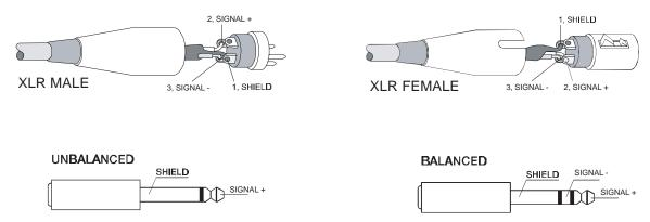
The following illustration shows the most important cable connections and their pin-assignment. A balanced wiring is to be preferred in each case.
