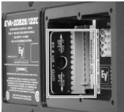
Figure 6.3: EVA input panel, with the switch card inserted to shade the lower HF element by 3 dB
