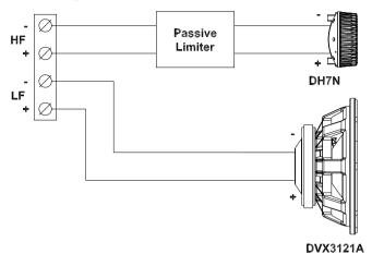
**Block Diagram (Passive):**Standard shipping configuration
