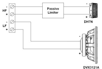
Block Diagram (passive): Standard shipping configuration
