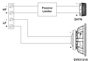
**Block Diagram (Passive):**Standard shipping configuration
