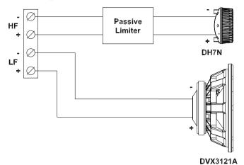
Block Diagram (passive): Standard shipping configuration
