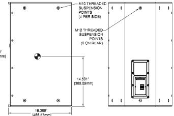
**EVF1152D43WLB 15" speaker 40x30 indoor white** EVF 15" / 2-way Full-range Systems; DVX woofer & DH7N driver (600 W cont.); 40° x 30°, EVCoat, white Order number **EVF1152D43WLB | F.01U.272.563**
