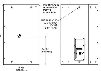
**EVF1152D96WLB 15"** speaker 90x60 indoor white EVF 15" / 2-way Full-range Systems; DVX woofer & DH7N driver (600 W cont.); 90° x 60°, EVCoat, white Order number **EVF1152D96WLB** | **F.01U.272.579**
