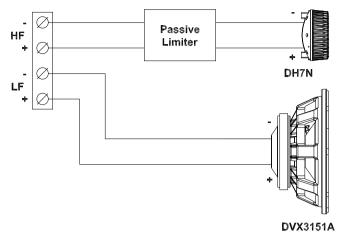
**Block Diagram (Passive):**Standard shipping configuration
