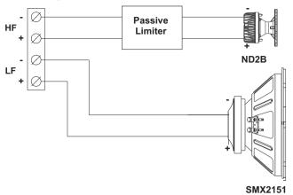
**Block Diagram (Passive):**Standard shipping configuration
