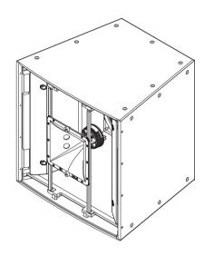
M10 suspension points for single hang (four shoulder eyebolts included) or an array (optional HRK or VRK kits).
