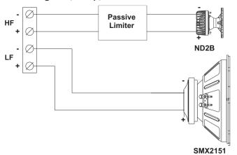
**Block Diagram (Passive):** Standard shipping configuration
