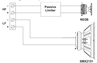
**Block Diagram (Passive):** Standard shipping configuration
