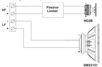
**Block Diagram (Passive):** Standard shipping configuration
