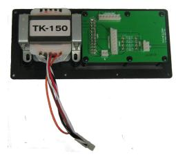
5. Secure the transformer mounting ears to the four (4) input panel bosses with the four (4) #10 screws provided. Carefully tighten the screws evenly in an X-cross pattern to avoid warping the plastic input panel.
