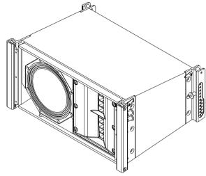
The XLE191-FG is a 2-way using a single 8-inch neodymium LF transducer and two neodymium 2-inch voice coil compression drivers with output combined through two Hydra waveform converters into a 90° x 10° waveguide.
