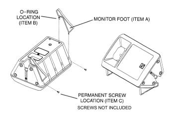
2. Permanently attach **feet** by using two (2) screws (The screws are not included with the kit. For more information, see Components.).
