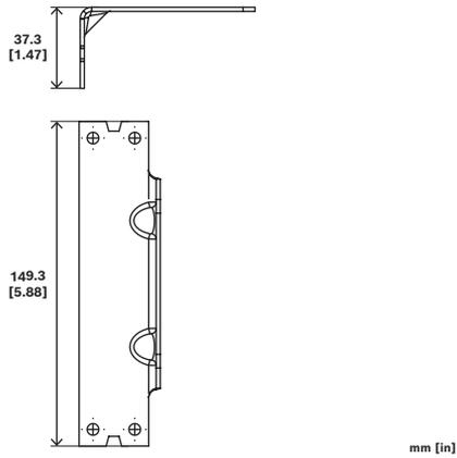
Fig. 1: Through hole bracket
