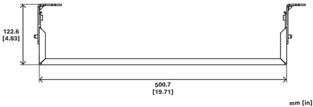
Fig. 3: U-bracket assembly
